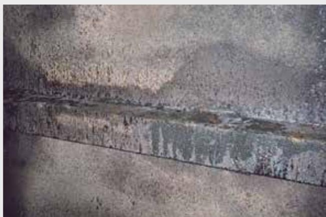
When this application was done the metal was damp, there were oxides on the surface of the metal. These rust marks are the result of
